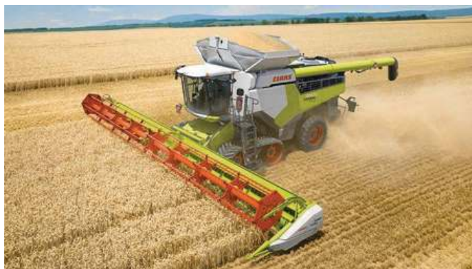
Claas Lexion 8900: 12 metre cutting head; throughput approaching 100 tonnes/hour; 16.2 litre MAN diesel engine developing 790 BHP; grain tank capacity 18 tonnes. GPS and laser guided; telematics delivering real-time data back to the farm office computer; on line diagnostics linked to an engineer in Germany. Cost: £400K - you could have a nice house for that....
